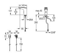
Touch: setting the sensor or features, by touching the sensor Battery: 6V Lithium CRP 2 - life time up to 4 years Mains operation: plug-in transformer 100-250VAC / 6VDC; VARIOconnect: single / multiple power supply, see accessories
